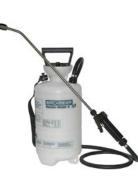
**CP4301** Impact resistant tank with Viton<sup>®</sup> seals, stainless steel pump rod and spray lance, safety valve and fanjet nozzle. Suitable for spray disinfection using Microsan<sup>®</sup> and Clensan<sup>®</sup>.
